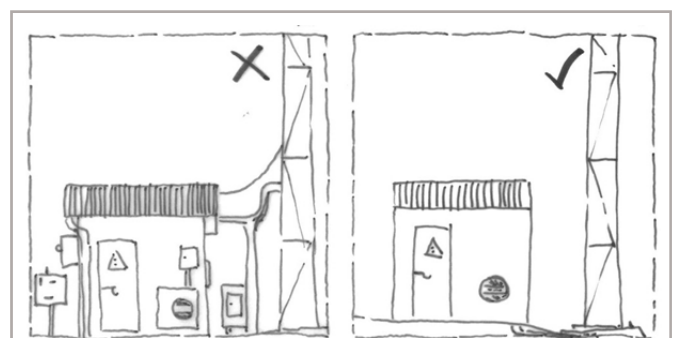
Accommodate mechanical equipment in container
